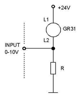
The resistance value of the resistor must be determined using Ohm's law. E.g. for voltage inputs 0-10 V a 500 Ohm resistor should be used (can be assembled in parallel with 2 pieces of 1 kOhm). When using the additional resistor, it is necessary to take account of the voltage drop across this resistor.
