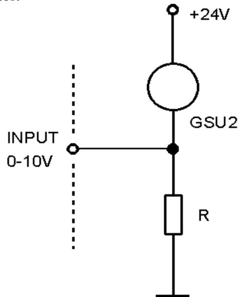
The resistor resistance value needs to be determined using Ohm's law. E.g. 500 Ohm resistor is suitable for 0-10 V voltage inputs (it can be connected in parallel of two 1 kOhm pcs). When using an optional resistor, it is necessary to take into account the voltage drop on this resistor.
