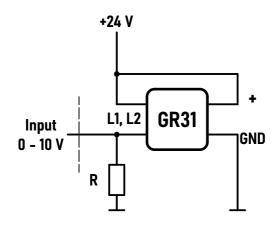
The resistance value of the resistor must be determined using Ohm's law. For example, for voltage inputs 0 to 10 V, a resistor of 500  $\Omega$  is suitable (can be assembled in parallel from 2 pieces of 1 k $\Omega$ ). When using an additional When using an additional resistor, the voltage drop across the resistor must be taken into account.
