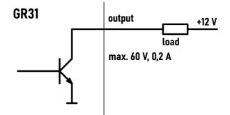
For output II, a jumper is available on the electronics board to select the quiescent state of the output transistor.
