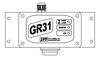
GR31 detectors are designed to detect explosive gases and vapors of flammable substances in indoor spaces such as boilers, process plants and facilities for converting cars to LPG, where ZONA2 environment is specified. Detectors use sensor operating on the absorption principle of infrared radiation to measure the gas concentration. The signal from the sensor is evaluated in the detector electronics, which controls the state of the detector outputs and signal lights.
